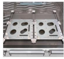
Option of placing more than one template on the work table, in order to increase productivity.
