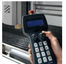
The hand-held terminal allows the operator to carry out the main machine operations with great ease and safety, as he can move away from the control panel when necessary.
