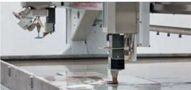
The software automatically adapts the number of cutting heads to suit the panels being created, to guarantee maximum productivity at all times without losing sight of flexibility requirements (one cutting head for pieces that are different from each other, or two for cutting several identical pieces simultaneously).
